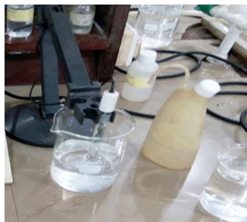
Figure 4. Testing for the Presence of Siloxane in Biogas.
