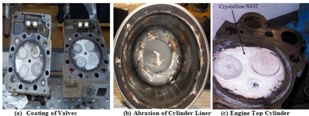
Figure 2. Effect of Siloxane on Engine Components [16-17].
